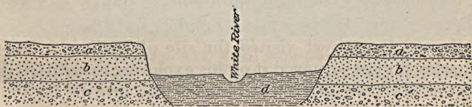
FIGURE 2.—Generalized section of White River valley at Kent, Wash., showing alluvium-filled depression in glacial deposits, including (a) Vashon drift, (b) Orting gravel, (c) Admiralty drift, and (d) deposits of present stream.
