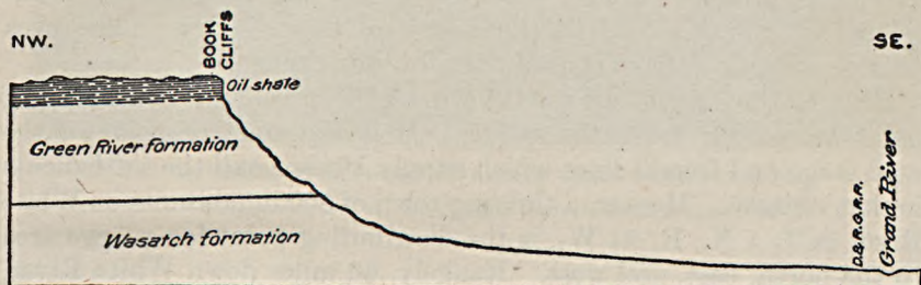
FIGURE 13.—Section from Grand River near Rulison, Colo., to the Book Cliffs on the north, showing the position of the oil shale.
