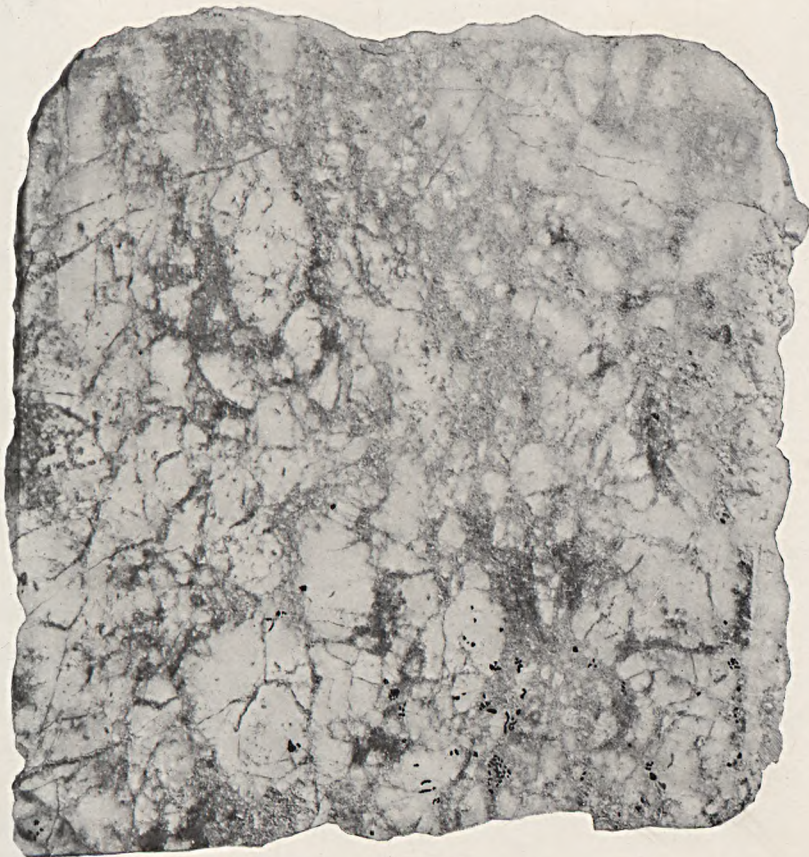
B. SAME SPECIMEN ENLARGED TWO DIAMETERS. SMALL BLACK SPECKS GOLD; GRAY MATERIAL STIBNITE.
