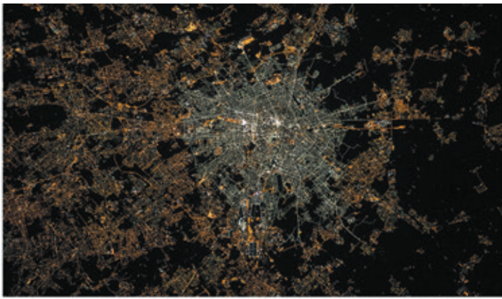
Milan in Italy replaced sodium street lighting with blue-rich white LED sources. City-centre illumination now looks brighter and bluer than in the suburbs.
