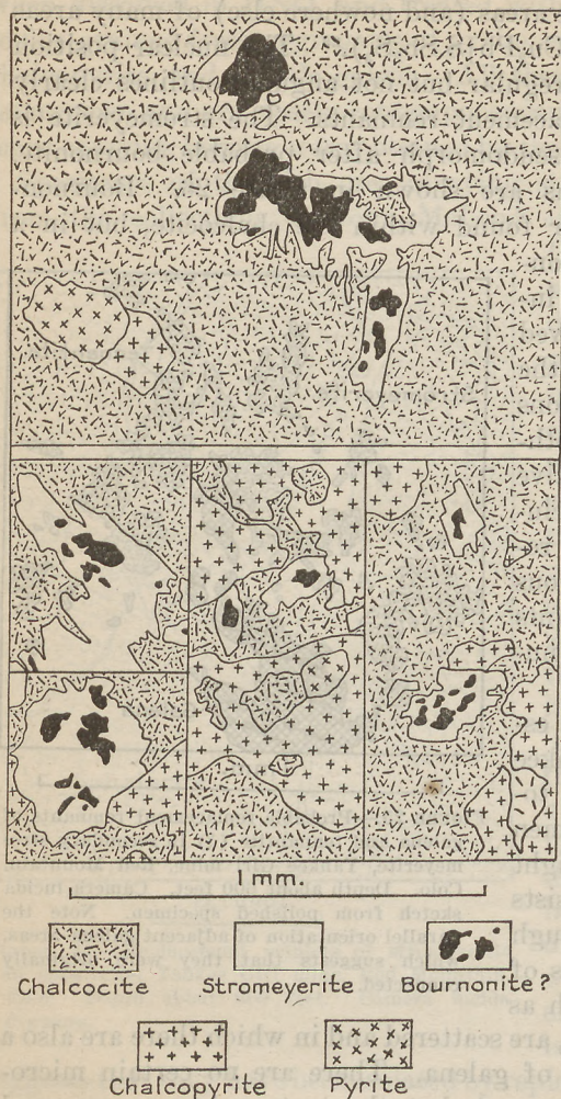
FIGURE 26.—Stromeyerite as a pseudomorphic replacement of bournonite (?), Yankee Girl mine, Red Mountain, Colo. Replacement remnants of bournonite (?), irregular but free from angularity, occur within the stromeyerite. Camera lucida sketches from polished specimens.
