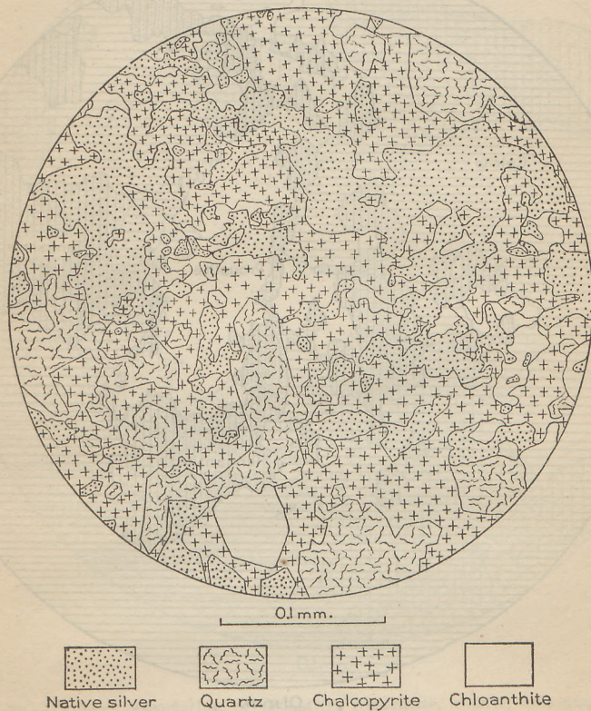
FIGURE 37.—Irregular primary intergrowths of native silver, chalcopyrite, chloanthite, and quartz, Monte Cristo mine, near Wickenburg, Ariz. Note that there are no indications that the silver has replaced other ore minerals. Camera lucida drawing from polished specimen.
