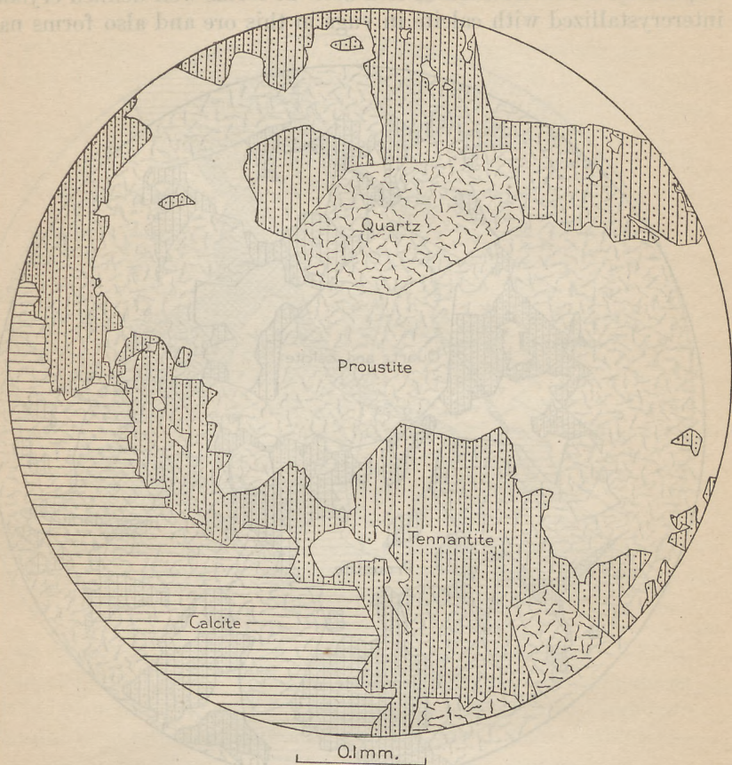
FIGURE 39.—Primary association of proustite, tennantite, calcite, and quartz, between 400 and 500 foot levels, Monte Cristo mine, near Wickenburg, Ariz. Note the nearly straight crystal faces common between proustite and tennantite; these indicate that neither mineral has replaced the other. Camera lucida drawing from polished specimen.
