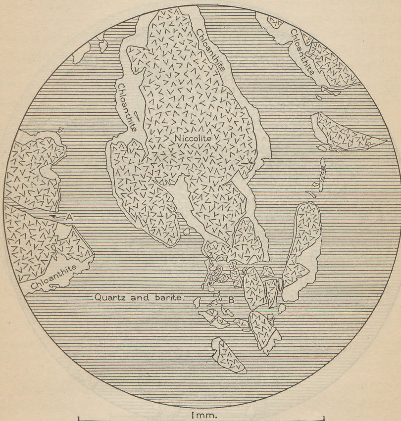
FIGURE 33.—Characteristic relations of niccolite, chloanthite, and calcite, Monte Cristo mine, near Wickenburg, Ariz. The chloanthite envelops the niccolite. Quartz and barite in turn envelop both; here and there veinlets of quartz and barite cut niccolite and chloanthite, as at A, or these minerals may embed fragments of niccolite and chloanthite, as shown at B. Camera lucida drawing from polished surface.
