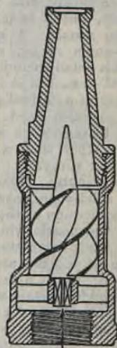
FIG. 3.—A large hollow-cone nozzle. (Courtesy of Schulte and Koerting Co.)
