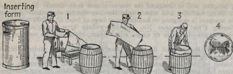
FIG. 101.—Method for inserting creped paper liners into barrels. (1) Insert the device into the lining as far as it will go. (2) Fold inwardly the ears formed by this operation and insert the lining and device into the barrel. (3) Fold the lining down over the chime of the barrel and remove the device. (4) The bottom of the lining lies smooth in the bottom of the barrel.
