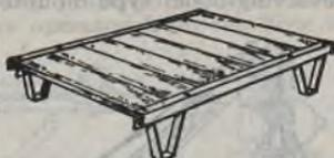
FIG. 22.—Standard type of skid platform.
