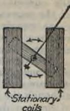
FIG. 98.—Dynamometer movement for voltage measurement.
