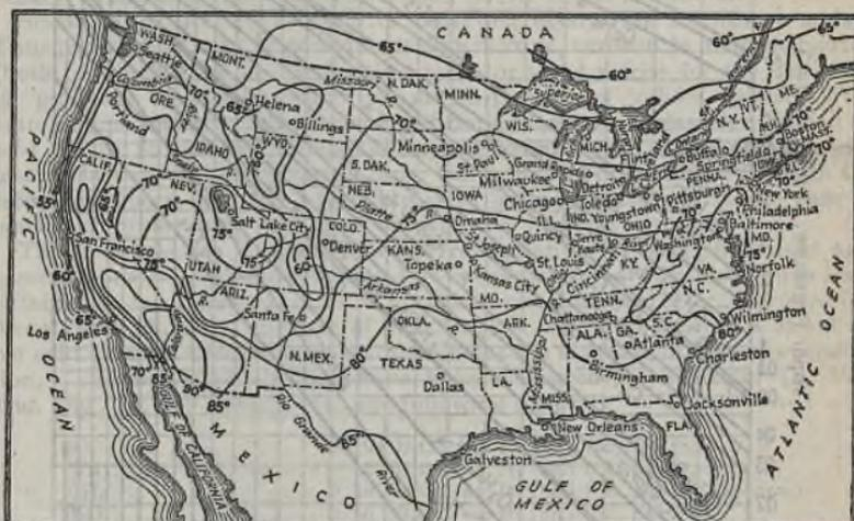
FIG. 15.—Surface-water temperatures (during summer months) in the United States. (Reprinted by permission from "Handbook of Mechanical Refrigeration," by H. J. Macintire, John Wiley & Sons.)
