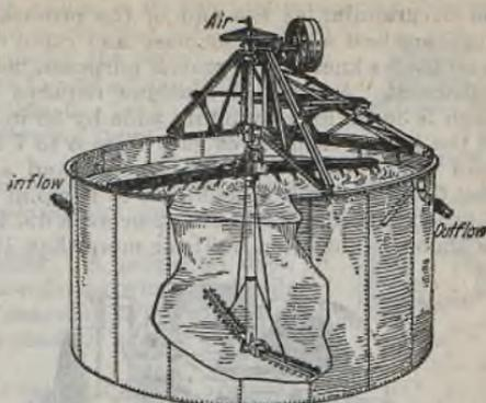
FIG. 16.—Air-lift agitator with scrapers.
