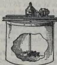
Fig. 27.—Simple turbine mixer.
