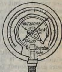
FIG. 23.—Bourdon-tube pressure indicator.
