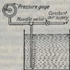
FIG. 60.—Back-pressure type liquid-level gage.
