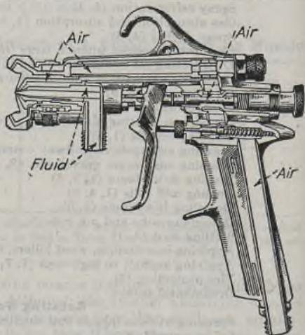
FIG. 9.—Typical spray gun. (Courtesy of DeVilbiss Co.)
