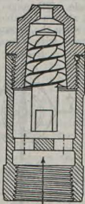
FIG. 2.—A small hollow-cone nozzle of the fixed spiral type. (Courtesy of Schulte and Koerting Co.)
