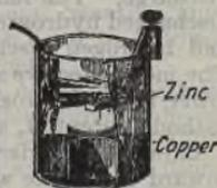
Fig. 3.—Gravity cell.
