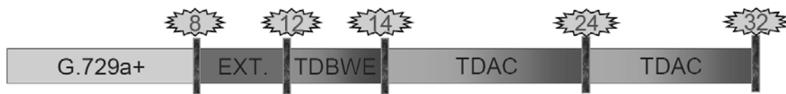
Fig. 2.10 Modes of G729.1 operation for various data rates in kbps
