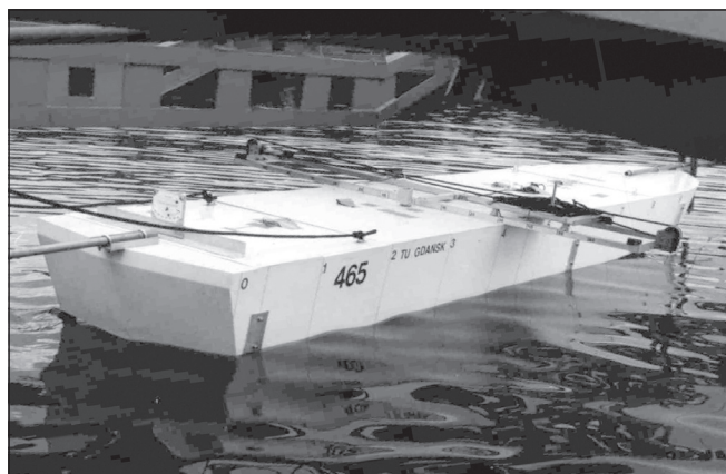
Model test of ship stability (photo: Mirosław Grygorowicz)
