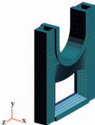
Fig. 2. Main bearing frame of Sulzer 7 RTA 84 C engine .
