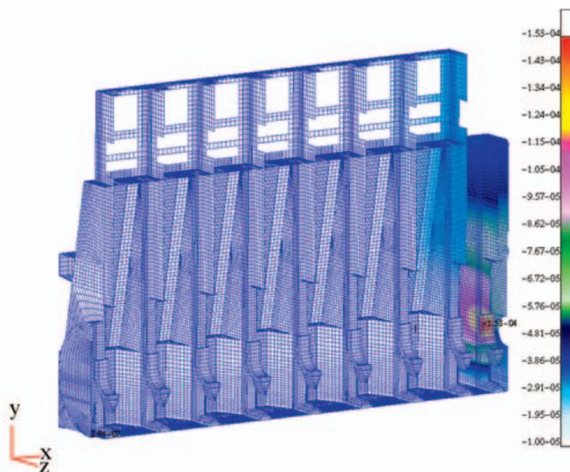
Fig. 7. Deformation of the main engine body under horizontal load applied to 1<sup>st</sup> main bearing .
