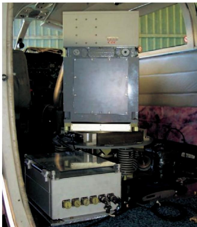
Fig. 1. The GT-1A gravimeter installed on Cessna 404 plane [12]
