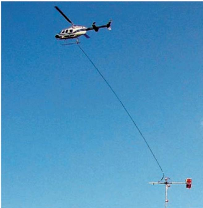
Fig. 16. The magnetic system on a helicopter with the magnetic sensor inside the gondola
