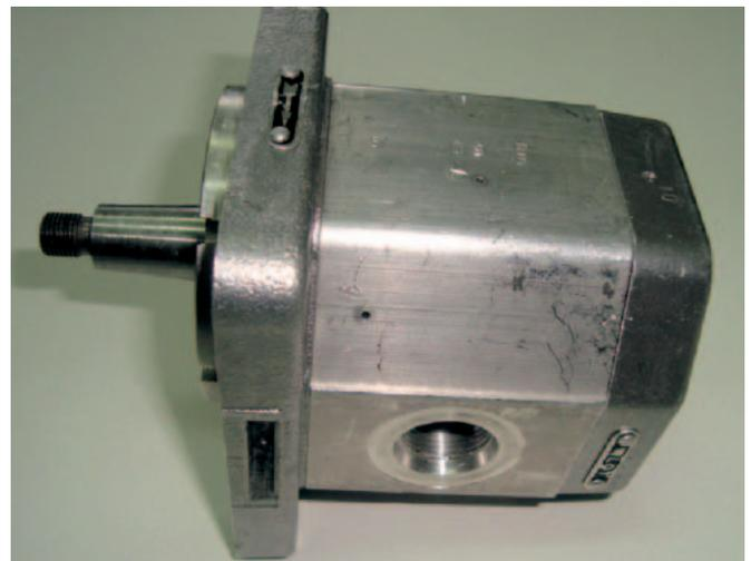
Fig. 4. Geared pump PZ2-K10 from Hydrotor company [19]
