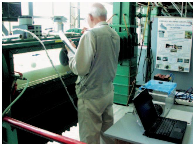
Photo 4. Research rig during ring thruster examination
