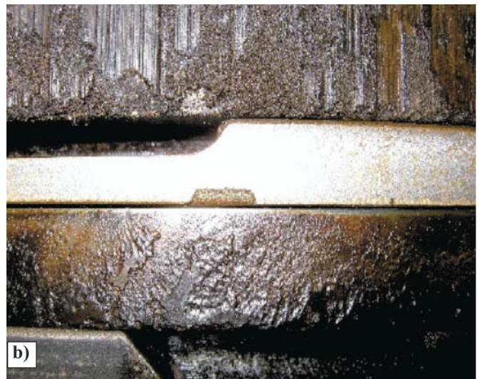
**Fig. 5.** Ring part of piston – the engine working on a biofuel produced on the basis of crude (not processed) palm oil.
