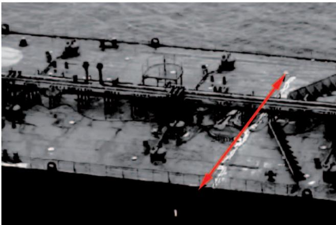
Fig. 2. Fatigue - cracked deck of the tanker Castor [4],
