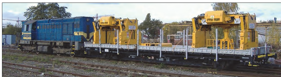
Rys. 9.42. Transport suwnic PTH-350/500 na wagonie [62]
