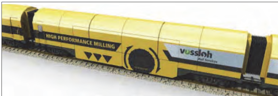
Rys. 8.45. Frezarka VMRM (Vossloh MFL Rail Milling) [82]
