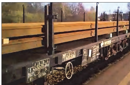
Rys. 9.1. Transport szyn na wagonach platformach
