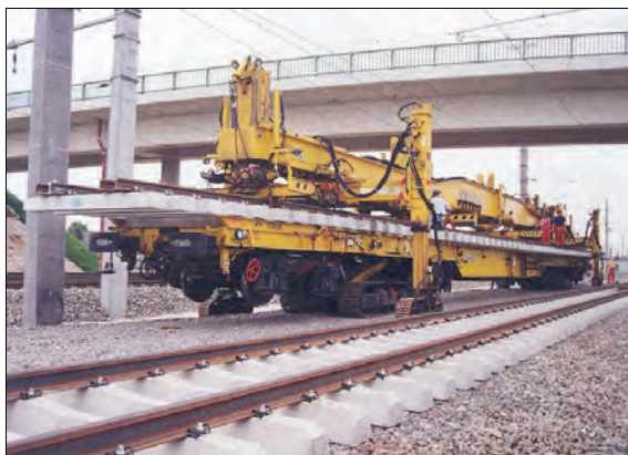
Rys. 10.41. Suwnica systemu WM500U firmy Plasser & Theurer [68]
