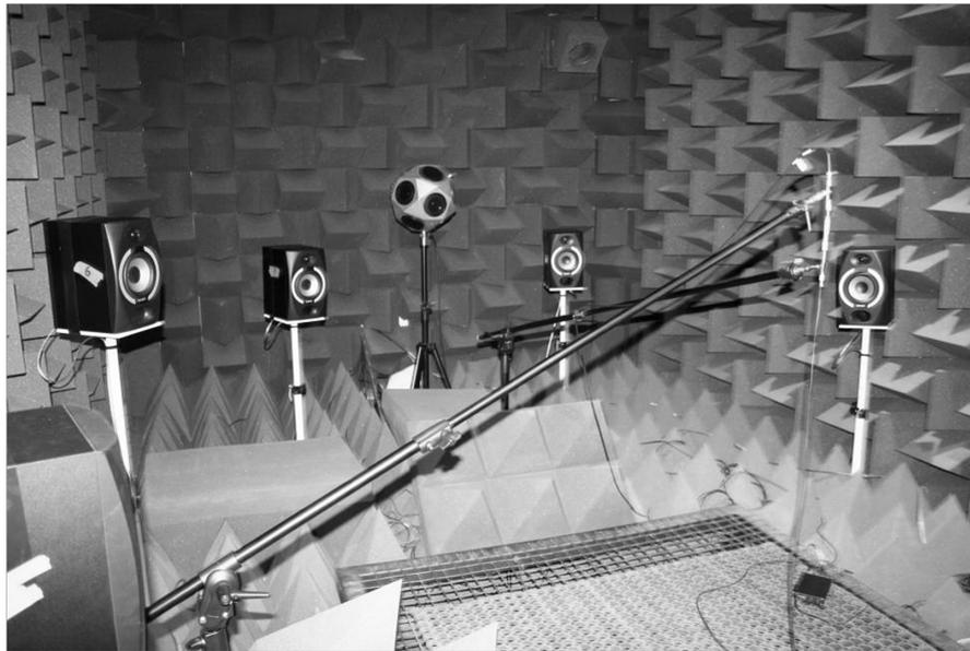
FIGURE 7.2: Photograph of the equipment employed for testing the sound recognition engine in simulated conditions
