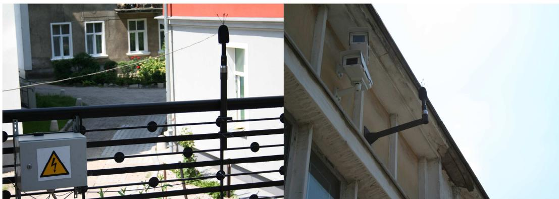
FIGURE 5.6: Example setup of microphones used for audio data acquisition
