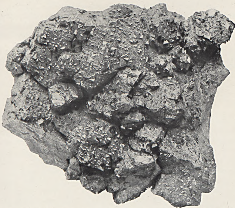
B. SPECIMEN OF CRYSTALLIZED CHALCOPYRITE WITH PARALLEL ORIENTATION ON SPHALERITE.
