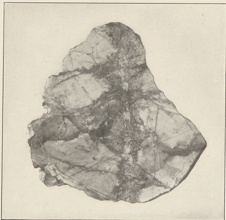
A. POLISHED SURFACE OF ALTERED LIMESTONE NEAR CASSITERITE LODE.
