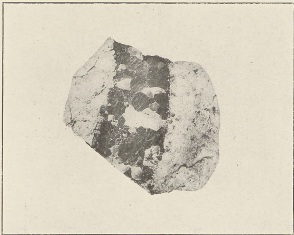
A. CASSITERITE AND WOLFRAMITE REPLACING CASSITERITE DIKE.
