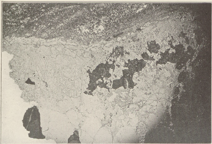
B. THIN SECTION OF CASSITERITE VEIN IN LIMESTONE NEAR CASSITERITE LODE.
