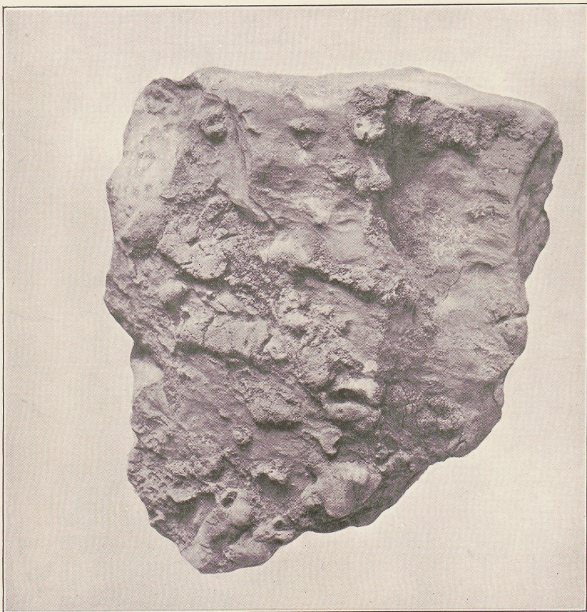
A. SPECIMEN OF GRANULAR CALCITE LIMESTONE WITH NODULES OF GRANULAR DOLOMITE IN RELIEF ON WEATHERED SURFACE.
