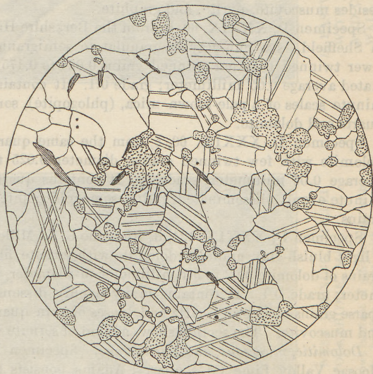
FIGURE 2.—Thin section of quartzose and micaceous twinned calcite rock from Hoosac Valley Lime Co.'s quarry, Adams, Mass. Enlarged 19.6 diameters. Dotted grains are quartz, shaded grains muscovite (white mica), black grains pyrite. Discarded in selecting stone for burning.
